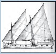
and stern, and propelled by oars or by sail in light winds. They were built to carry a heavy cannon in the bow, flanked by smaller cannon and swivel guns, and measured about 70 feet long. Twenty double-manned oars on each side required at least 80 seamen who stood upright to row. Troops from the Continental Line were drafted to serve as marines.
